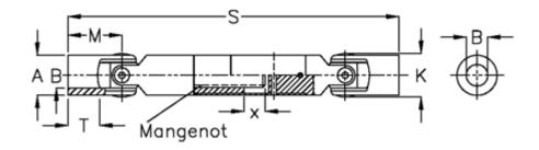
$\begin{array}{lll} A & = 63 \\ B \ H7 & = 40 \\ Longitudinal \ ribs = 6x36x42 \\ M & = 83 \\ MD \ max \ N \ m & = 450 \\ s & = 585 \\ T & = 50 \\ \end{array}$
